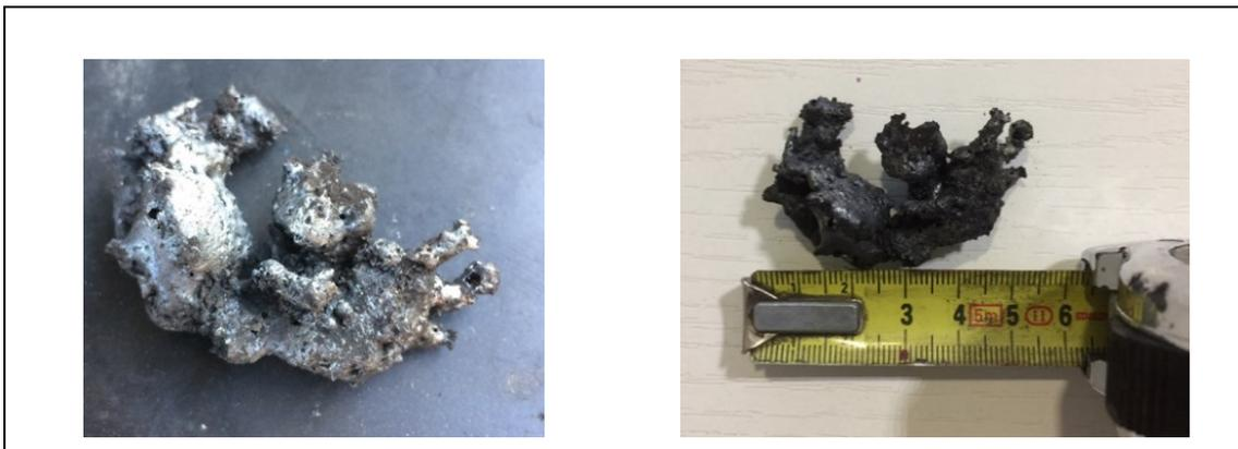
Figure 2. 13: Fragment of molten ash present in the reactor combustion area.
