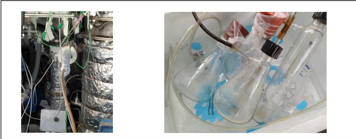
Figure 2. 8: Experimental setup for the analysis of the tar concentration in the syngas
