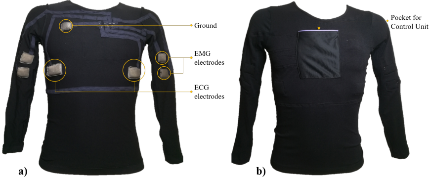
Figure 2.2. SWEET shirt sensing unit: (a) internal view with textile electrodes and connections, (b) external view.
