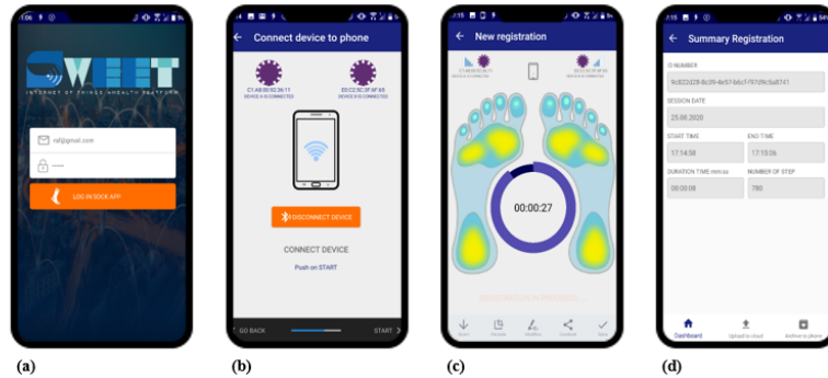
Figure 3.4. SWEET App main frames: (a) login; (b) unit connection; (c) signal recording; (d) results summary.
