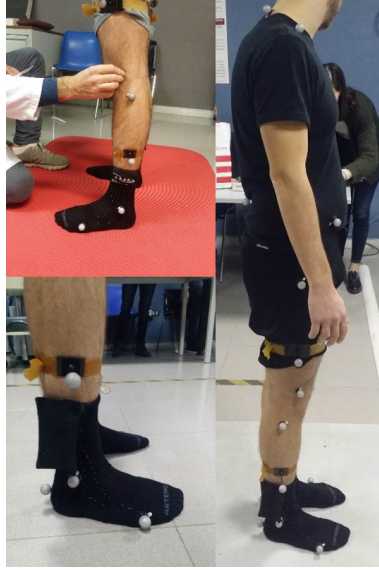
Figure 3.5. Subject equipped with both systems: SWEET Sock and reflective markers.
