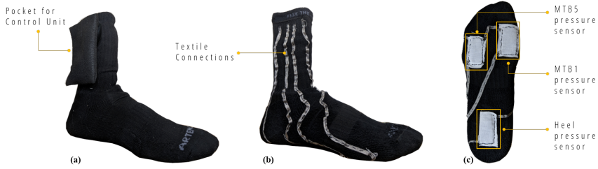
Figure 3.2. SWEET Sock sensing unit: (a) external view; (b) internal view of textile connections; (c) textile pressure sensors.
