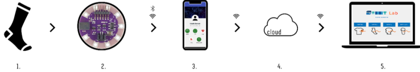
Figure 3.1. System Architecture: (1) SWEET Sock-Textile Unit; (2) SWEET Sock-Control Unit; (3) SWEET App; (4) Web Server; (5) SWEET Lab.
