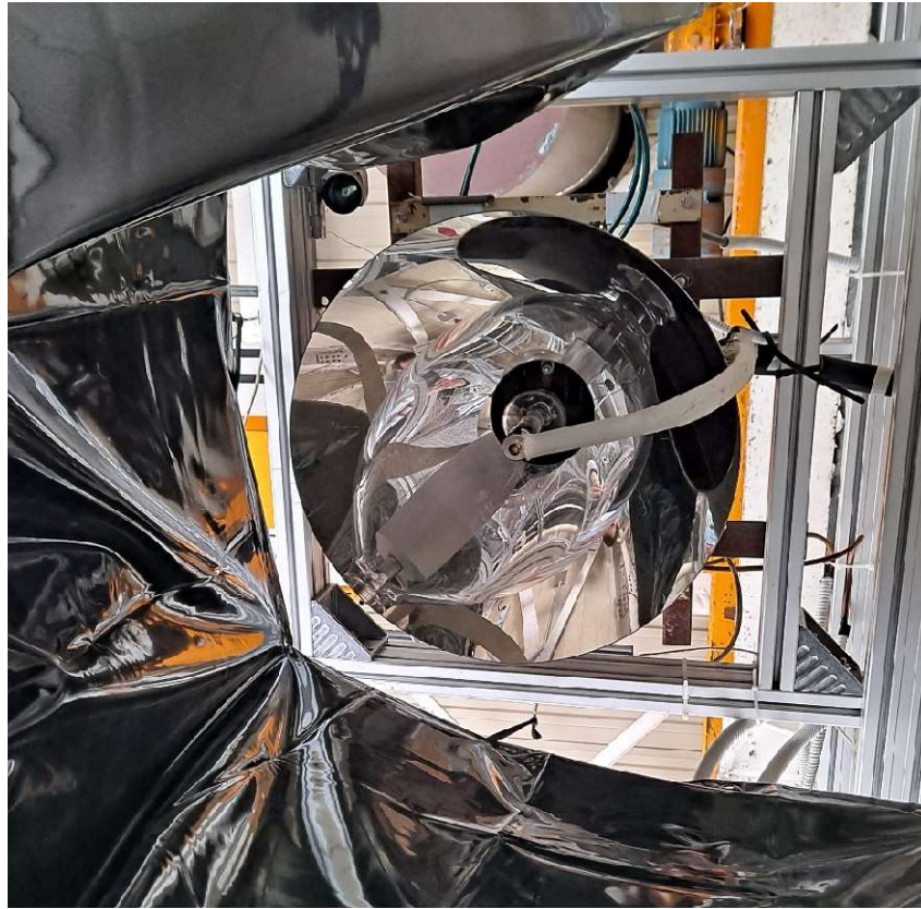
Figure IV.3 Photo of the 10 kW el solar simulator.
