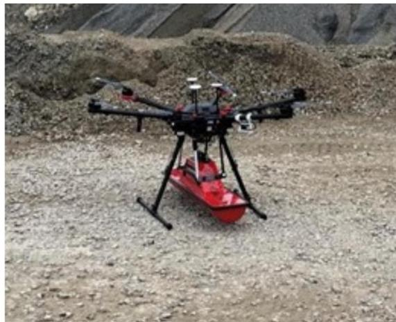
**Figure 5.** Picture of the UAV GPR System developed by the Dyrecta Lab., Conversano, Italy.
