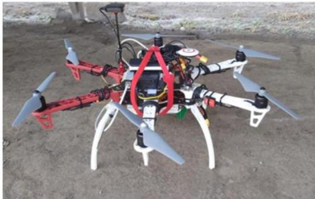
**Figure 2.** Picture of the UAV GPR system developed at the Department of Industrial Engineering (DII) of University of Naples “Federico II”.
