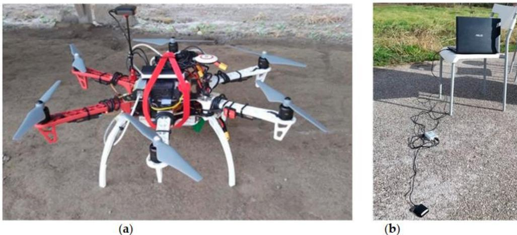
**Figure 19.** M-UAV radar imaging system (System HI): (a) DJI F550 hexacopter with on-board equipment; (b) ground-based GPS station.
