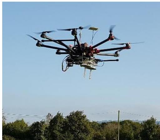
**Figure 1.** Picture of the UAV-GPR system developed at University of Oviedo, Gijon, Spain.
