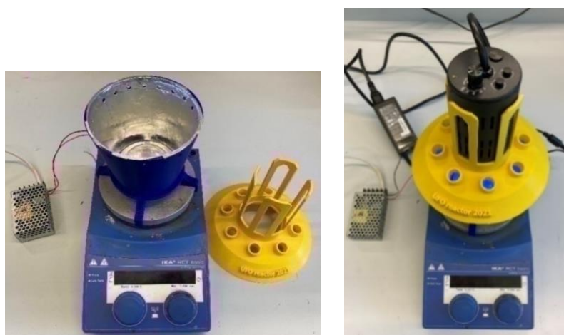
Figure S2 Pictures of the assembled reactor equipped with a Kessil lamp (365 nm).
