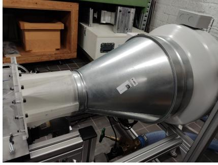
**Figure B.5.** Picture of the connection component between the blower (on the right) and the air duct (on the left).
