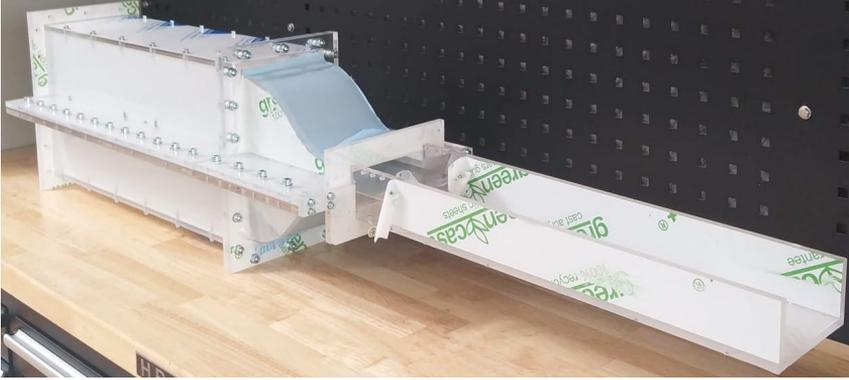
**Figure B.3.** Picture of the experiment core realized in Plexiglas. The test section is also shown (on the right).
