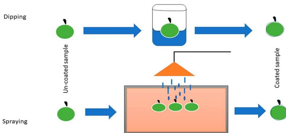
Figure 3. Dipping and spraying technique to apply coating on the product (Khan et al., 2021)
