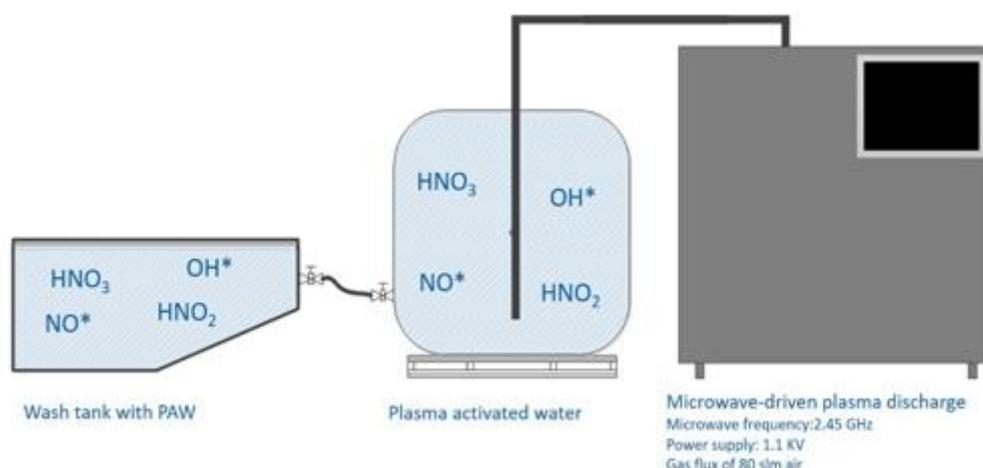
Figure 1 Schematic drawing of the PAW producing system
