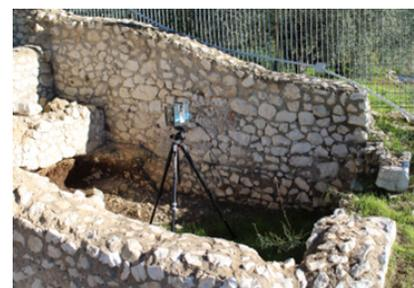
Fig. 78 \_ Laser scanner Faro Focus 3D s150
