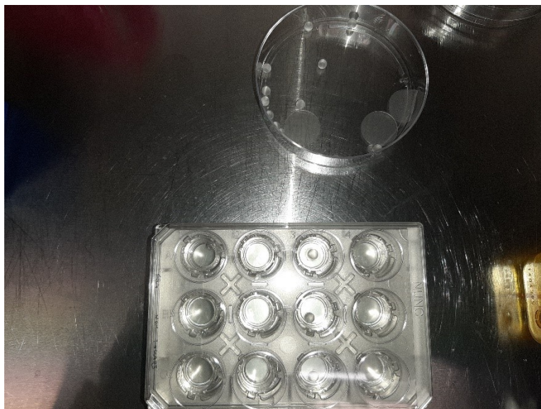
Figure 4.3.2.2: Image of UV 3D printed disks (up) for cell adhesion tests and multiwell with UV 3D printed spherical components (down) for cell viability tests. No unpolymerized resin is visible.
