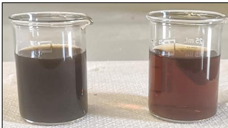
Figure 5.6 – Aqueous phases generated by the HTL process and separated by L-L extraction (left) or centrifuge (right).
