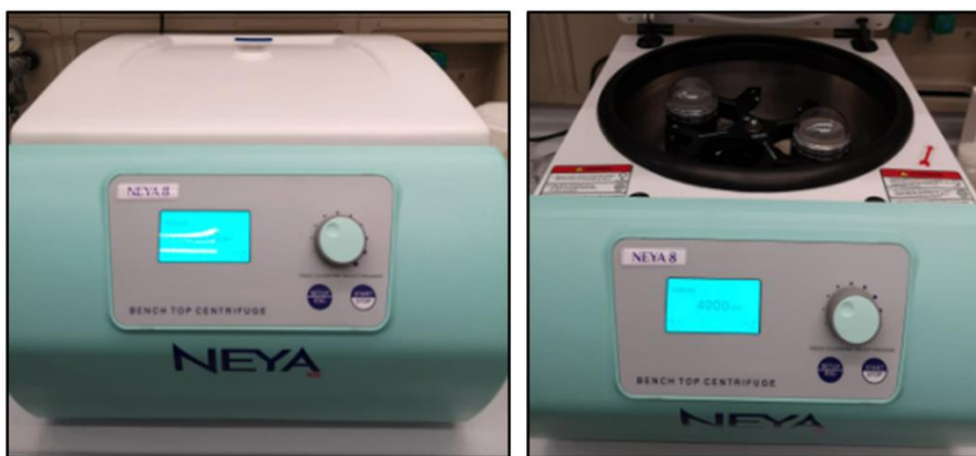
Figure 2.14 – NEYA 8 BASIC ventilated centrifuge used for the separation of bio-oil from the aqueous phase.
