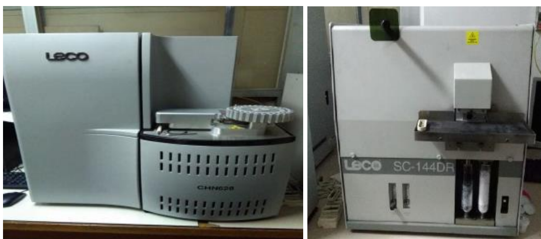
Figure 2.2 – LECO CHN628 (a-left) and LECO SC-144DR (b-right) analysers.
