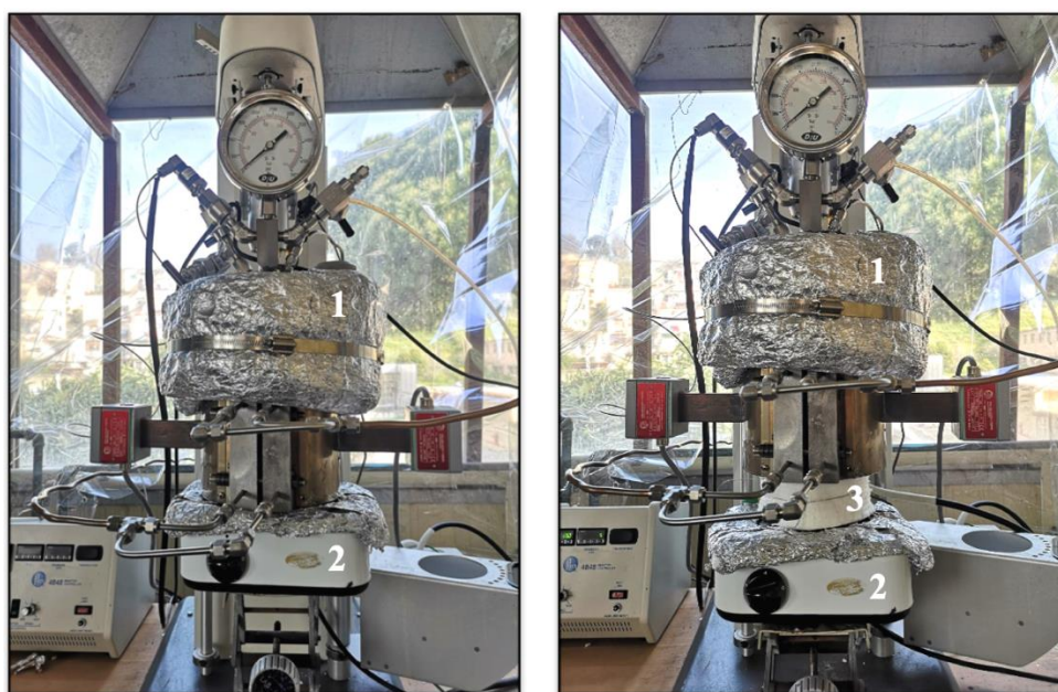
Figure 2.12 – Left) configuration B and Right) configuration C of the experimental apparatus for HTL tests; 1) rock wool insulation, 2) heating plate 3) insulated heating bands.
