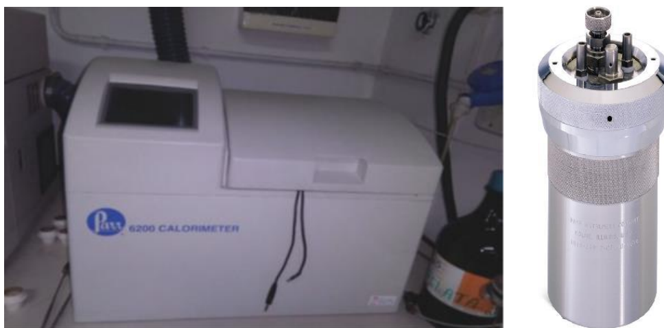
Figure 2.3 – Parr 6200 calorimeter (a-left) and sealed calorimeter bomb (b-right).
