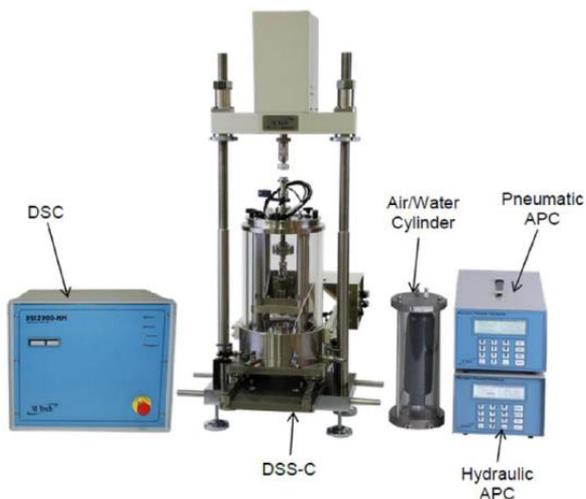
**Figure 5-36:** Basic system components of Cyclic Simple Shear (CSS) apparatus with confining pressure (Mele, 2020).
