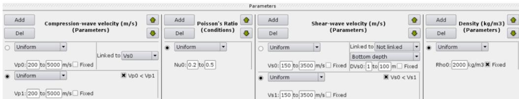
**Figure 6-2:** Example of parameter input panel for inversion.
