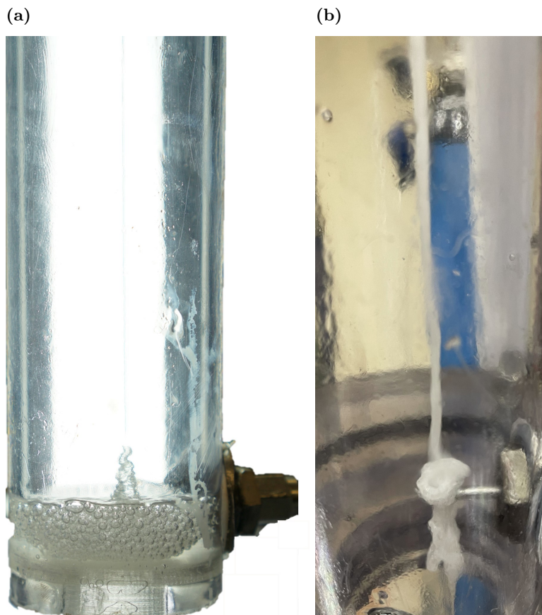
Figure 2.12: Typical experiment with perforated obstacle configuration (2.12a), and without obstacle (2.12b). In both cases the sensor is inserted from the right.
