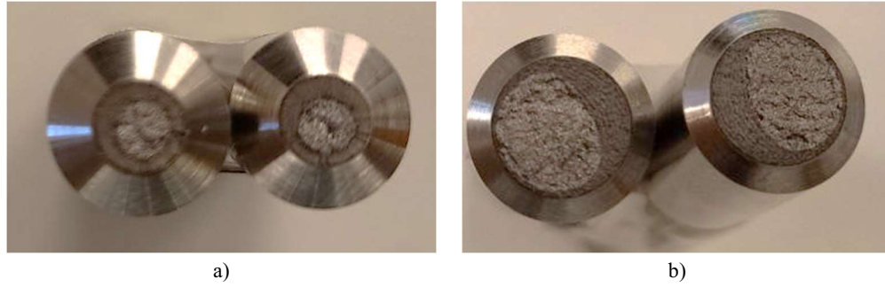
Figure 4.4 Macroscopical fracture surfaces for statically tested specimens: a) T5001 and b) T7501.
