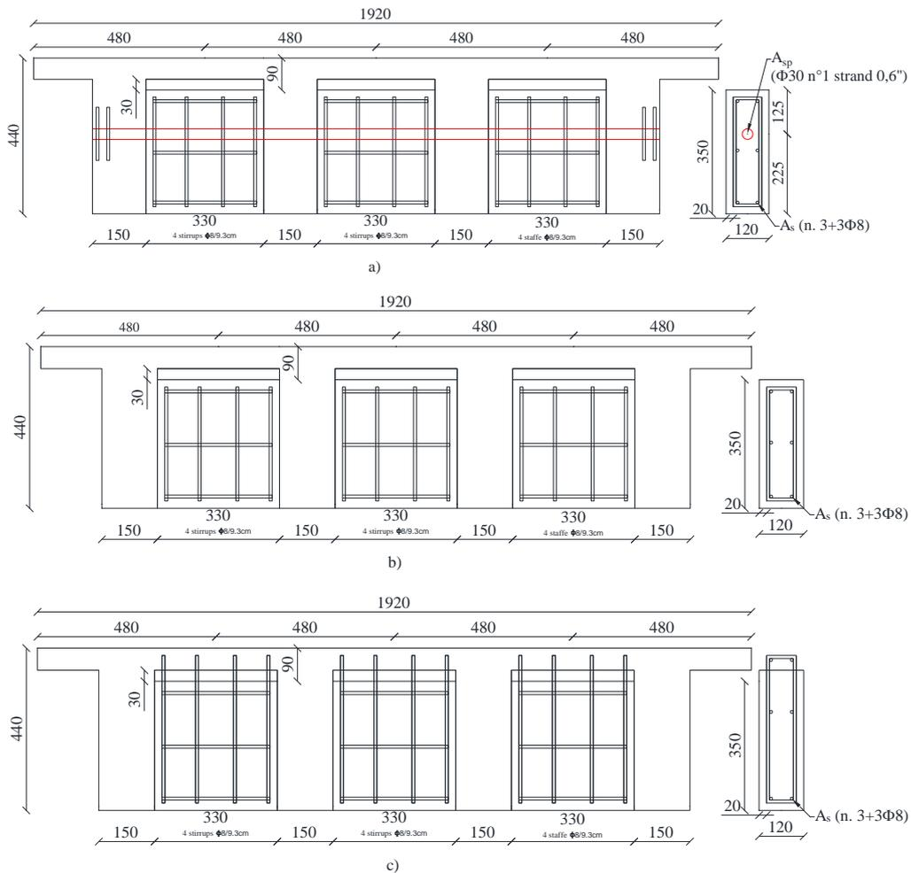
**Figure 51.** Bridge deck and cross girders cross sections considering: (a) prestressed cross girders separated from RC slab; (b) cross girders separated from RC slab; (c) cross girders connected to RC slab.
