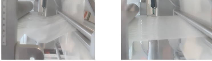
Figure 4.9. Peel measurements with (left panel) and without (right panel) waves formation. Right image represents the condition where measurements of peel force are reliable.
