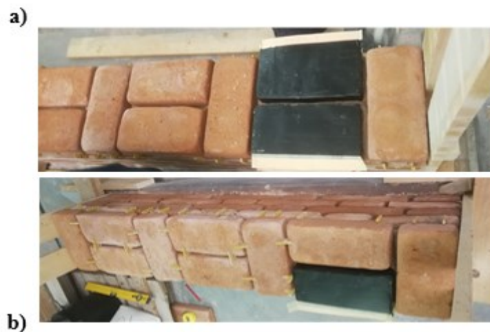
Figure 3. Smart bricks pattern for diagonal compression test: a) Intact; b) Deteriorated
