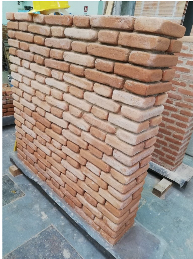
Figure 2. Pictures of specimens to be tested under (a) simple compression and (b) diagonal compression
