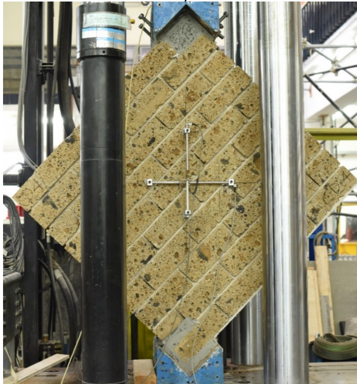
Figure 9. Experimental setups of specimens subjected to diagonal compression in configuration (a) intact and (b) deteriorated.
