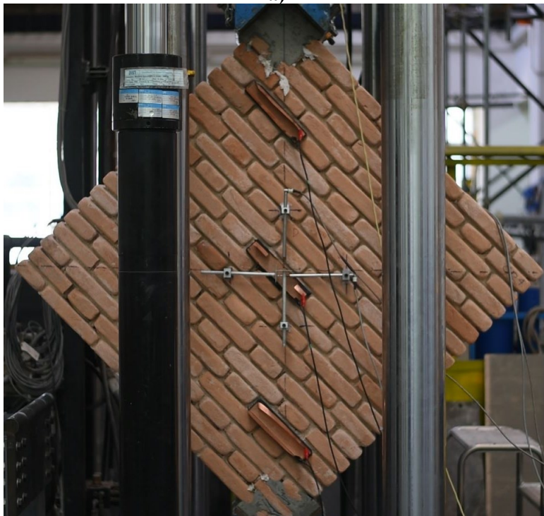
Figure 4. Masonry bond pattern for diagonal compression test with smart bricks for configuration: a) intact; b) deteriorated
