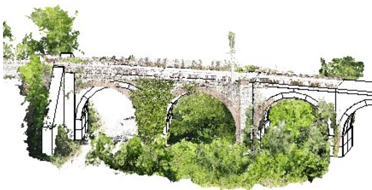
Figure 3.23 - BIM modeling (using Revit software) starting from the point cloud.
