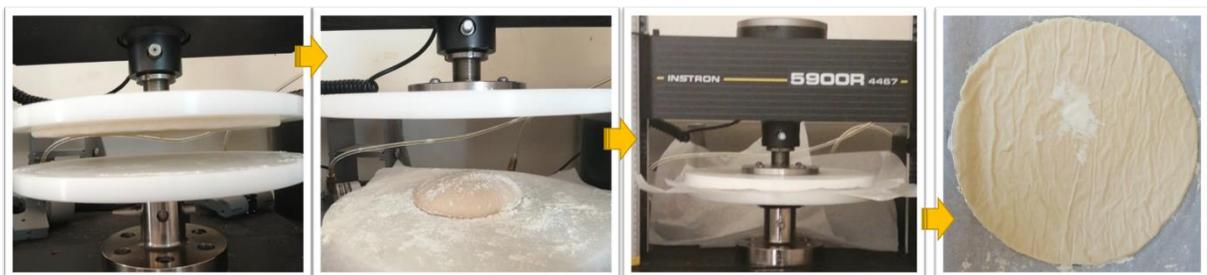
**Figure 1.S2**– Flow chart of compression of pizza dough in the two mounted plates ( $\varnothing$  30 cm) of the dynamometer (Instron, mod. 5900R, USA).
