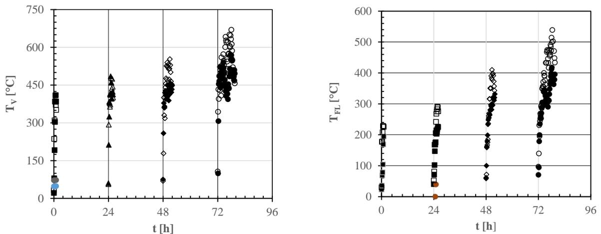
1410 **Figure 2:** Time (t) course of the oven vault ( $T_V$ : **left**) and floor ( $T_{FL}$ : **right**) temperatures as measured
