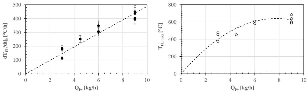
1456 **Figure 4:** Effect of firewood feed rate (Q<sub>fw</sub>) on (left) the derivate of the oven floor temperature with
