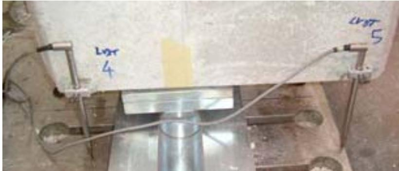
Figure 2.16 –LVDTs to measure hinge rotations
