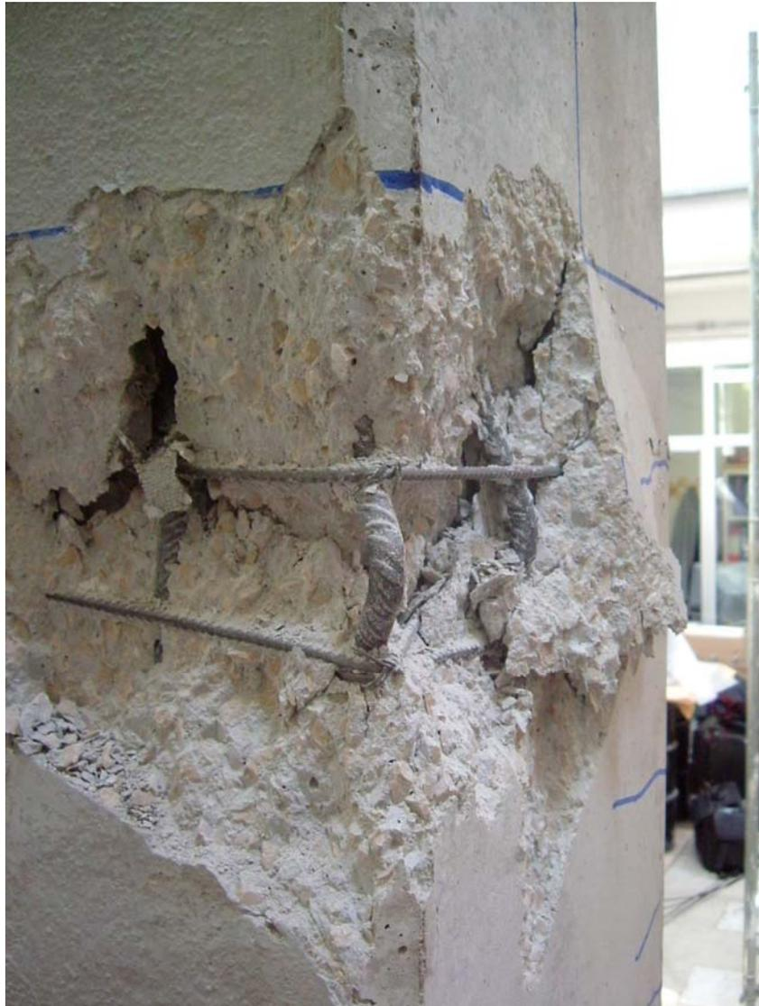
*Figure 4.3 –Buckling of the outermost bar (U2)*
