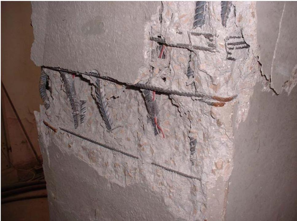
*Figure 4.2 – Compressed Bars Buckling and Concrete Cover Spalling (U1)*
