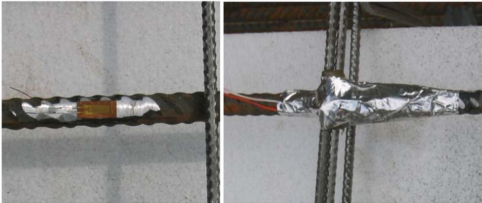
*Figure 2.12 –Strain Gauge on the internal steel reinforcement*
