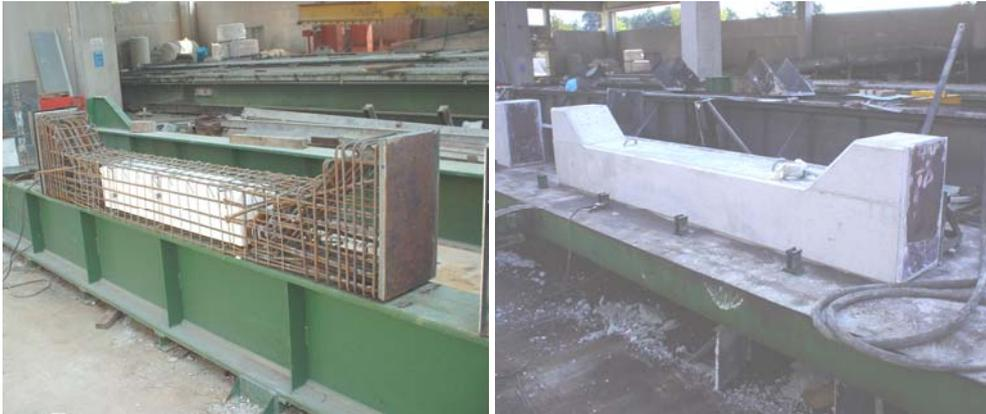
Figure 2.5 – Specimen: cage ready for concrete pouring and after concrete curing
