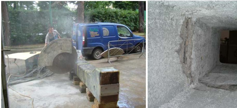
*Figure 2.33 –Inside view of the hollow portion after failure (S1)*
