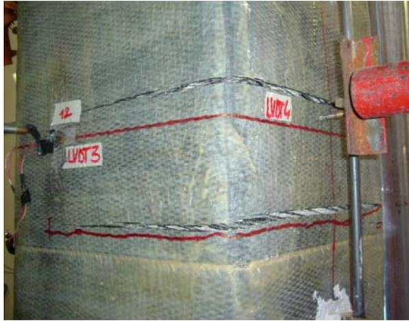
Figure 4.5 –Wide cracks opening in tension side (S3)
