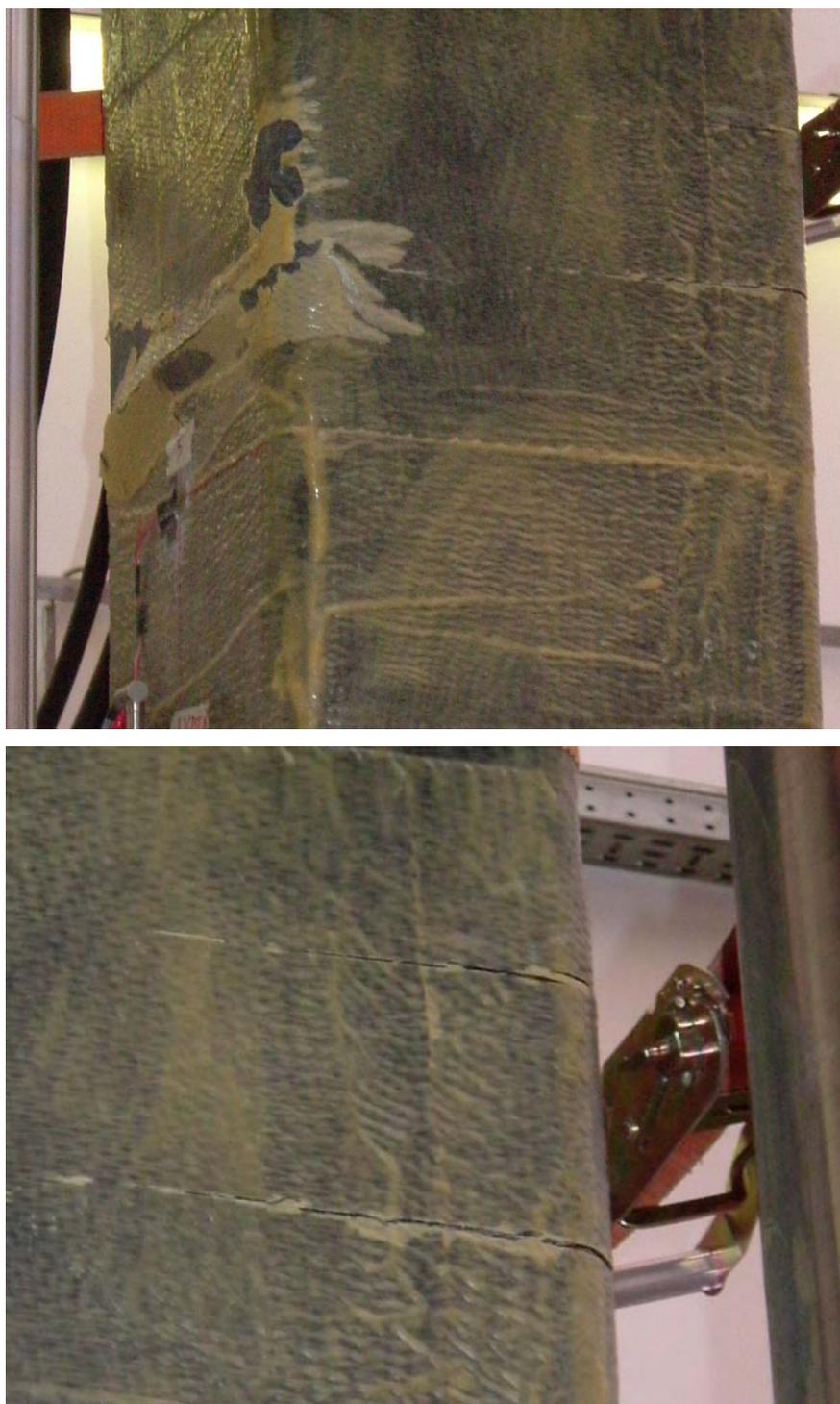
*Figure 2.38 –Bulge of FRP wraps and crack opening at failure (S2)*
