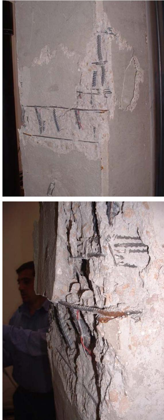
*Figure 2.17 –Crushed wall and steel reinforcement buckling (U1)*
