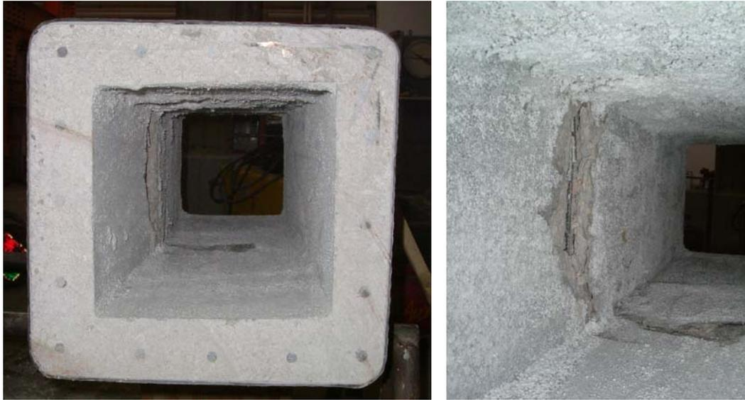
Figure 4.7 –Failed portion of the specimen after test (S1)
