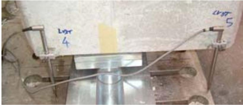
Figure 2.16 –LVDTs to measure hinge rotations
