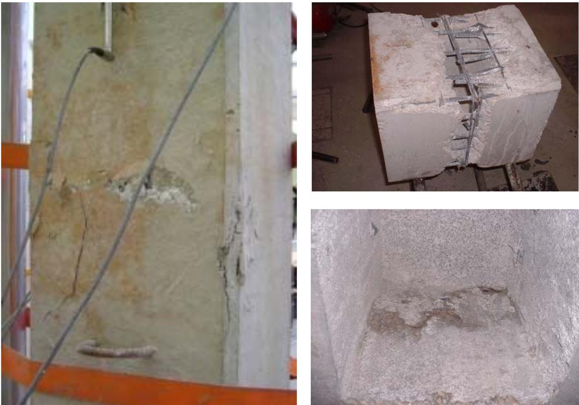
*Figure 2.25 –Crushed wall and steel reinforcement buckling (U3)*
