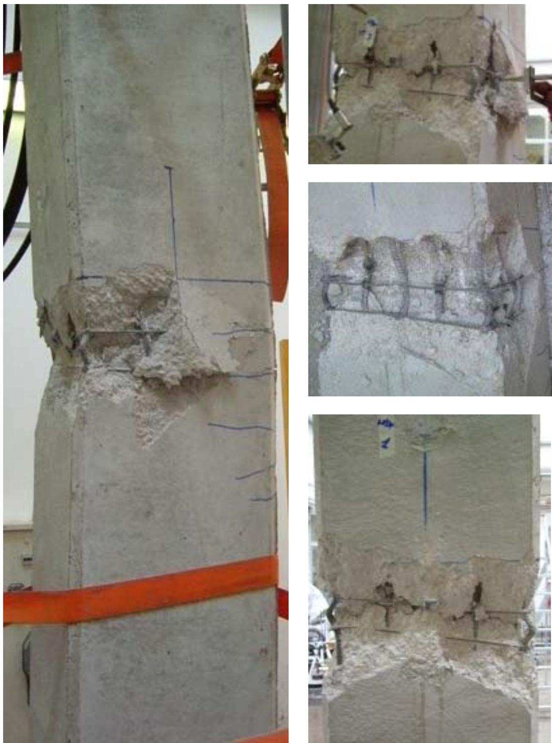
*Figure 2.21 –Crushed wall and steel reinforcement buckling (U2)*
