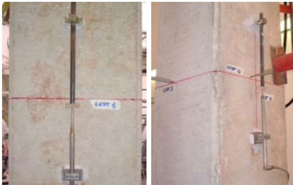
*Figure 2.14 –LVDTs on the hollow portion*
