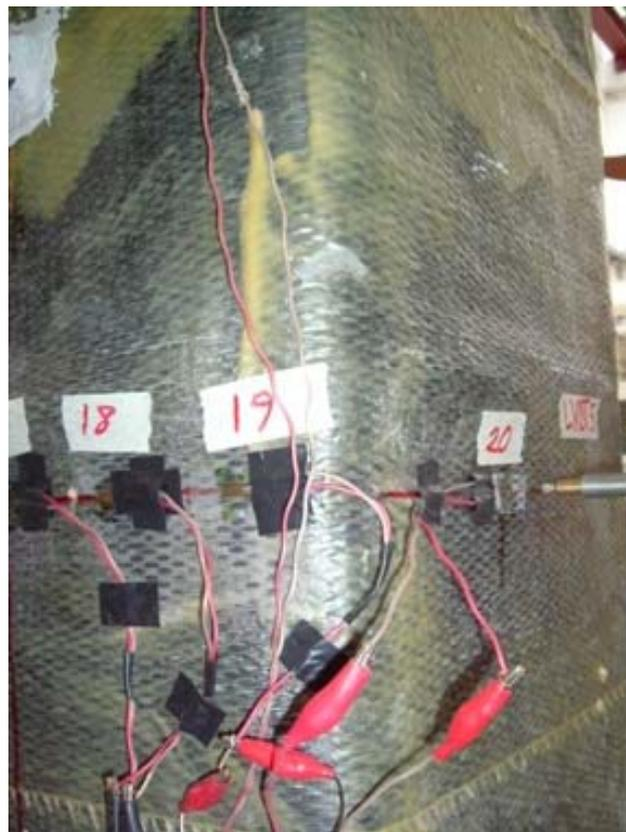
Figure 2.29 – Detail: Strain Gauges measuring FRP strains over the corner (S1)
