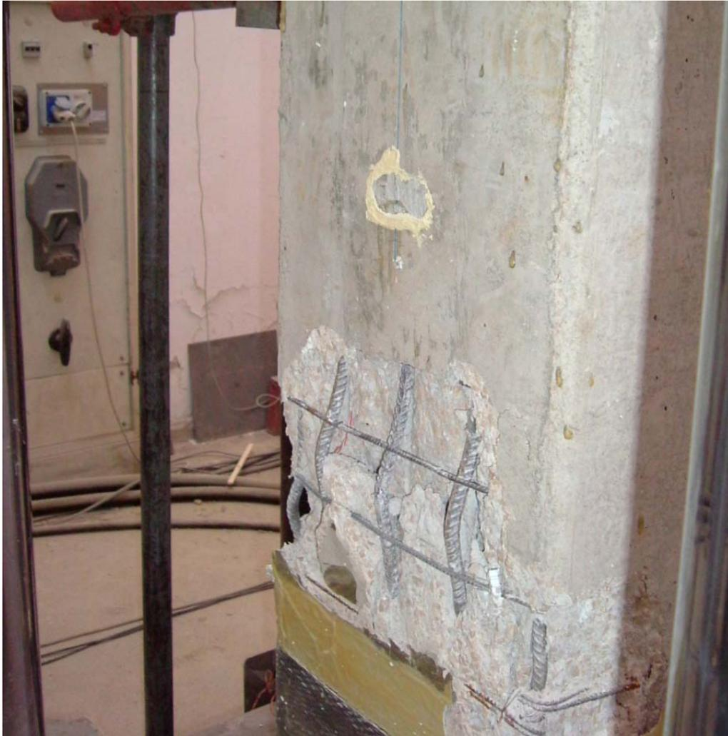
*Figure 2.8 – Column U0 at failure*
