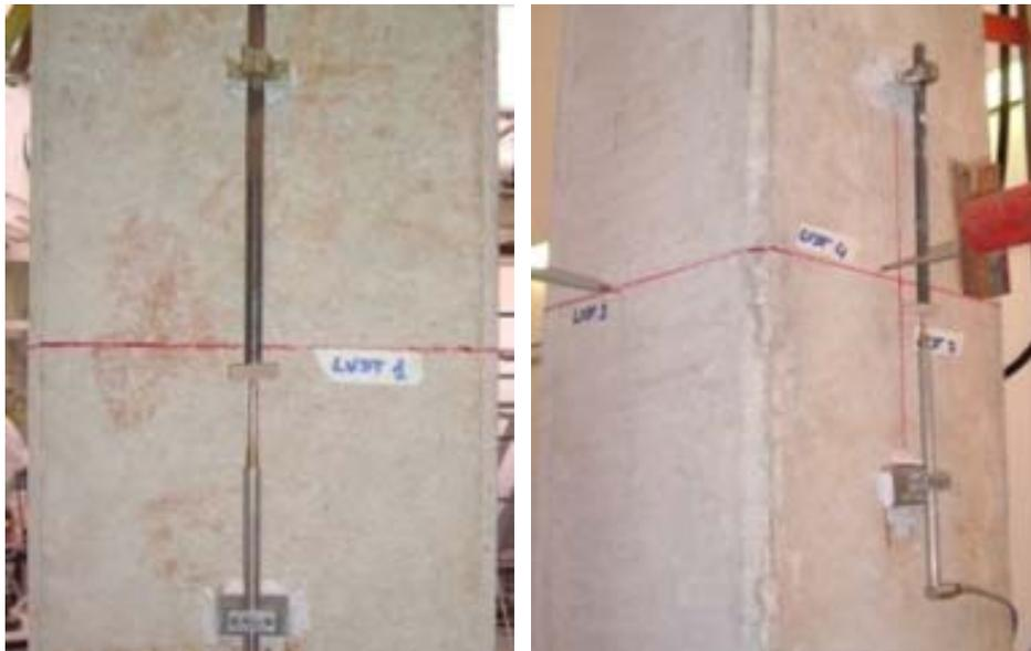
*Figure 2.14 –LVDTs on the hollow portion*
