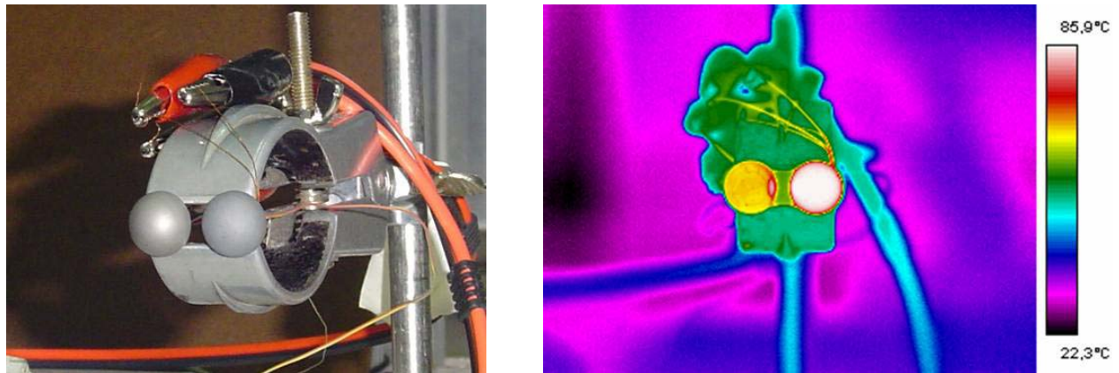
Figure 63 (a) Comparison between two UHTC specimens: the right one has been exposed to the high enthalpy flow; the left one is virgin and (b) infrared image of the two specimens
