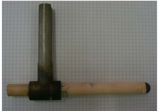
Figure 90 (a) UHTC specimen and (b) the model, after the first experimental test
