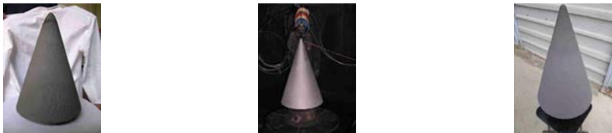
Figure 3 (a) C/SiC nose cap technology demonstrator, (b) ZrB 2 -SiC deposition into Plasma SprayChamber and (c) Technology demonstrator made of C/SiC substrate and ZrB 2 -SiC coating
