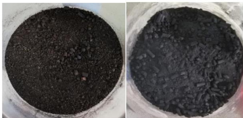
Figure 4-2. From left Biochar at 285 °C and Biochar at 450°C
