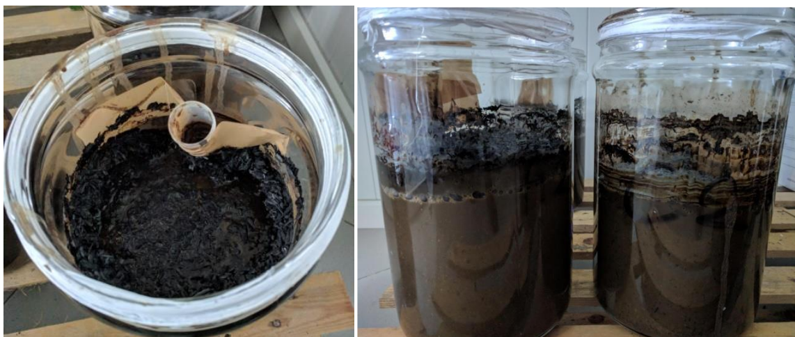
Figure 4-5. From the left. Formation of biochar crust in the sample 1B. Volume reduction followed the storage period.
