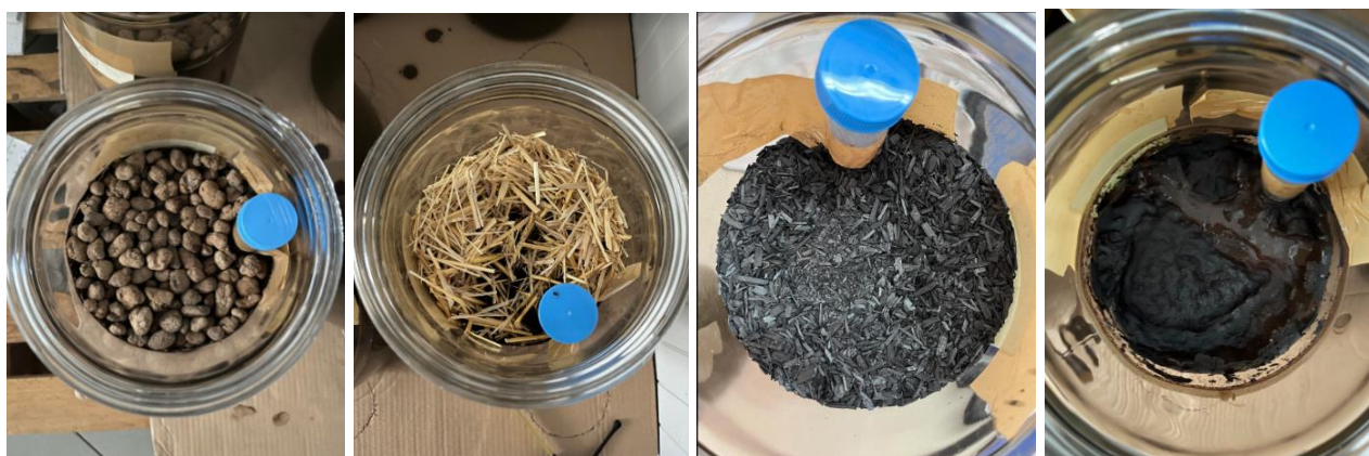
Figure 5-1 Tested cover on digestate surface. From the left: clay, straw, biochar, control, respectively
