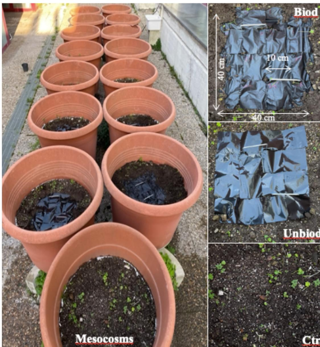
**Fig. 2.1** Experimental mesocosms (left) and details of soils covered by un-biodegradable and biodegradable plastic sheets and uncovered soils (right).
