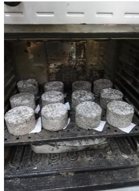
Figure 53 – Specimens took off the oven at 60°C after three days of curing time.
