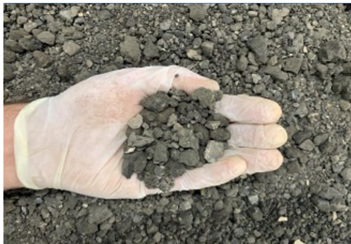
Figure 5 – The RAP employed into the asphalt mixtures.
