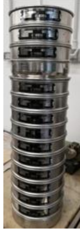
Figure 48 – EN 2332 sieves arranged with decreasing dimensions from top to bottom of the mesh opening.
