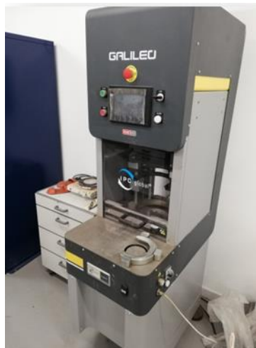
Figure 52 – Superpave Gyratory in the Laboratorio di Strade Luigi Tocchetti – University of Naples Federico II.
