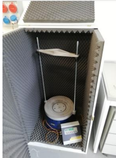
Figure 49 – Vibrating Screen in the Laboratorio di Strade Luigi Tocchetti – University of Naples Federico II
