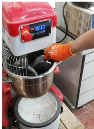
Figure 51 – Heavy Duty Lab Mixer in the Laboratorio di Strade Luigi Tocchetti – University of Naples Federico II.
