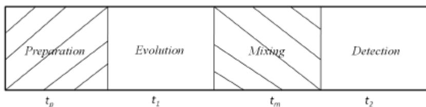
**Figure 2.10** General Schematic of 2-D NMR experiments to detect multiple-quantum coherences.
