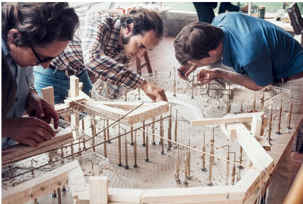
Fig. 10 Frei Otto Atelier Warmbronn, costruzione del modello sospeso per il progetto della Multihalle di Mannheim, scale 1 : 100, ca. 1973. © Frei Otto Archives, Carlfried Mutschler + Partners Archives. © saai | Archive for Architecture and Engineering at Karlsruhe Institute of Technology (KIT)
