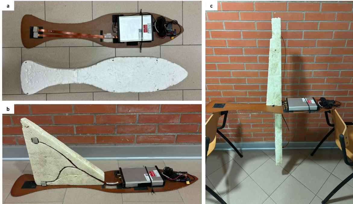
Figure 3.2. MFAM custom bird solutions. a) Configuration with sensors maintained on the same horizontal plane; b) Vertical gradient arrangement, with baseline of 0.25 m; c) Vertical gradient arrangement, with baseline of 1 m.
