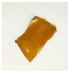
Fig. 2. Sheet of the biodegradable material obtained by drying the hydrogels produced with CH/R1 or CH/R2 at 3/7 mass ratio.
