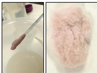
Fig.2. Poly- \gamma -glutamic acid produced by PB5390 and PB5523 B. subtilis strains with E-medium after methanol precipitation (left panel) and after dialysis and freeze drying (right panel).
