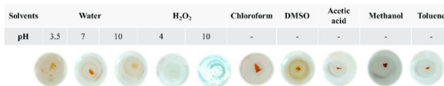
Figure 2. Images of CHR1(2/8) sample immersed in distilled water at different pH values (3.5, 7.0, and 10.0), or in 30% ( w/v ) of H 2 O 2 at different pH 4.0 and 10.0, or in different organic solvents.
