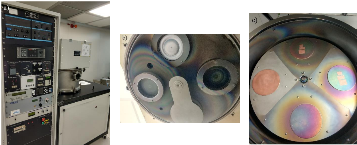
Figure 1.13 Sputtering deposition system. The sputtering apparatus (a). Sputtering targets (b). Rotating supporting disc with four sample holders (c).
