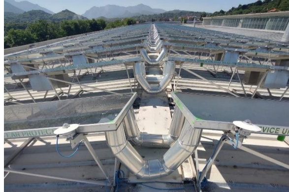
Figure 4.7 Arrangement of the two pyranometers for the second measurements campaign.
