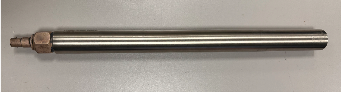
Figure 3.2: 1" inch \varnothing \times 25 cm length cylindrical 10 bars pressure ^3\text{He} -filled proportional counter with stainless steel housing. The same model and dimensions as those used for underground neutron background measurement, ^{13}\text{C}(\alpha, n)^{16}\text{O} direct cross-section measurement [63], and in the SHADES project.
