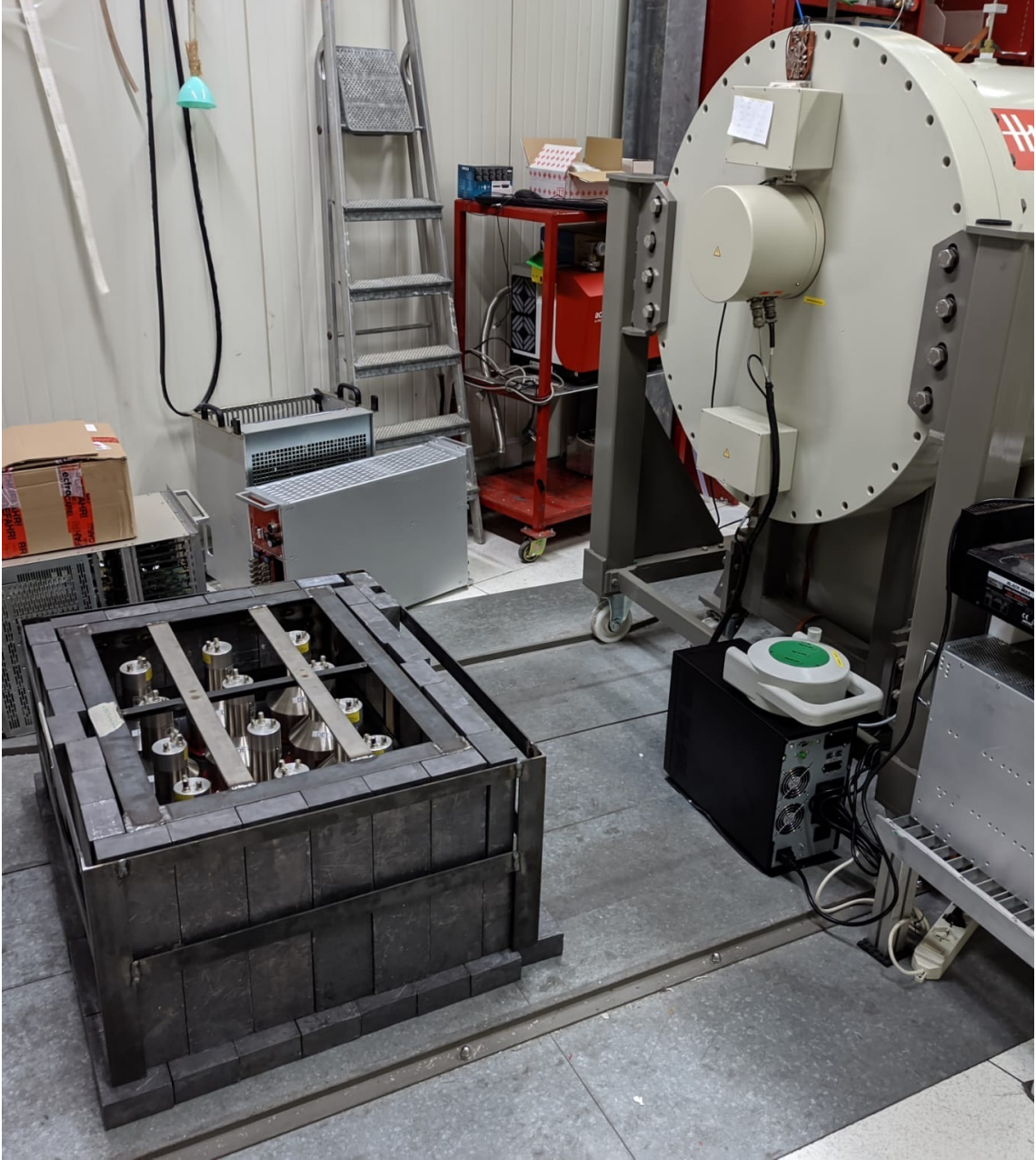
Figure 4.2: EJ-309 scintillators arrangement inside lead shielding in the LUNA-400 accelerator room at LNGS (Hall-A) during the internal background measurement.
