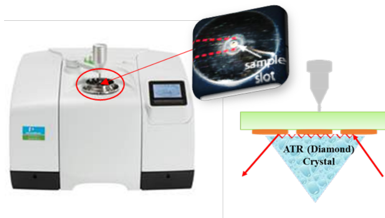
Figure 5.1. (a) The PerkinElmer Spectrum 3 FT-IR spectrometer with ATR module (b) Detailed schematic of the ATR measuring system.
