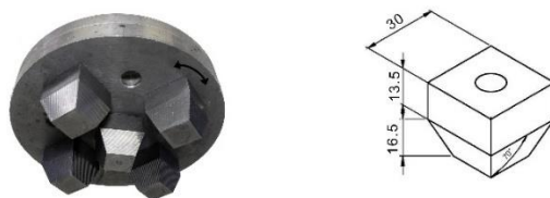
Figure 1. AIP for punching tests: Geometric design. All measurements are in mm.
