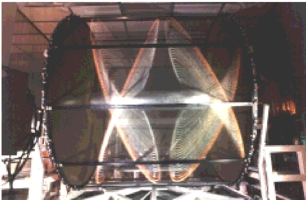
Figure 2.7: The KLOE drift chamber at the end of the wire stringing.
