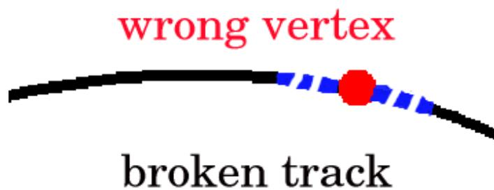
Figure 5.8: Vertex obtained by a kaon broken track.
