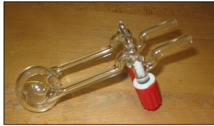
Fig 3.13 Glass bulb with fitting valve used as reference radon source
