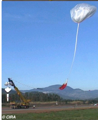
Dynamic launch of the balloon. The payload hangs from a crane-like device ready to be released.
