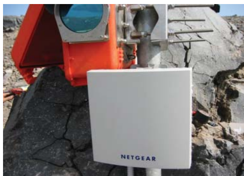
Fig. 6. Directional antenna for wi-fi data transmission to Lipari Island.
