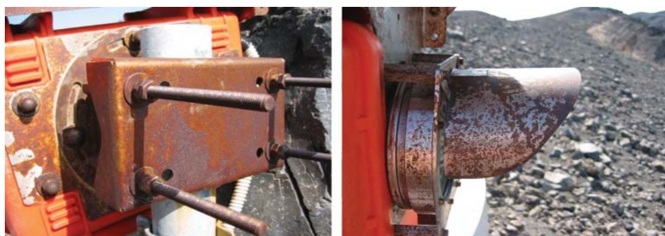
Fig. 10. Gas corrosion effects at Vulcano station.
