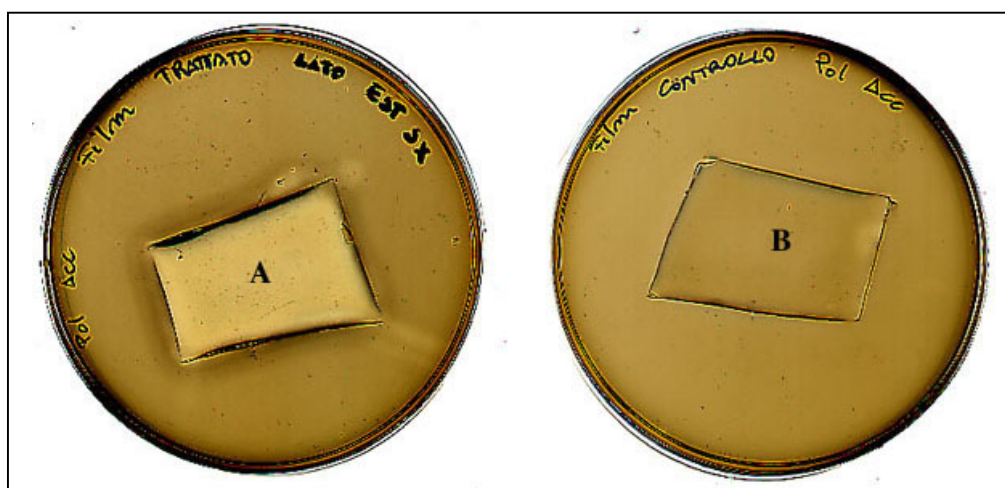
Fig. 3.7 - Antimicrobial activity of the PE-OPA film coated in the industrial plant with PPBAC 32Y solution at 6400 AU/ml against the indicator strain Listeria monocytogenes V7. A , treated film; B untreated film.
