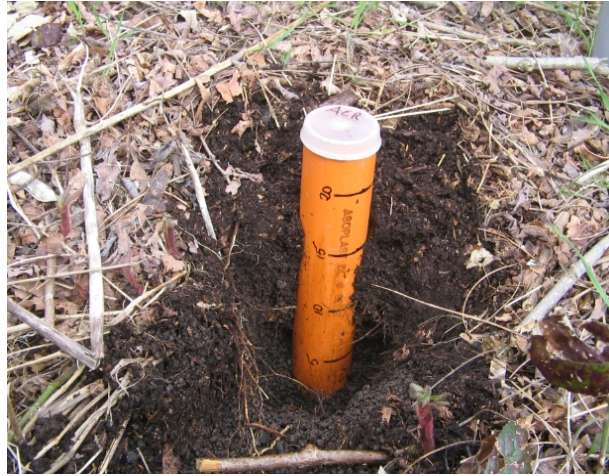
Figure 9. The mineral soil was sampled until a depth of 15 cm when possible using a corer with the surface of 25 cm 2 .
