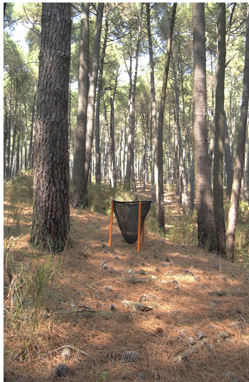
Figure 6. Cannello mangano (CM). Details of litter trap in the 96-year-old Stone pine ( Pinus pinea L.) monoculture on the most southern side of Mount Vesuvius.
