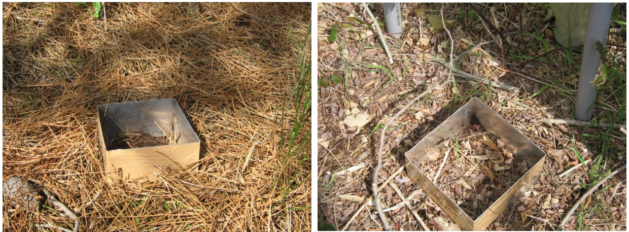
Figure 8. A quadratic sampler of 400 cm 2 (20 x 20cm) for collecting the material in the organic layer in the stands studied: details in Corsican pine stands (to the left) and in Black locust stand (to the right).
