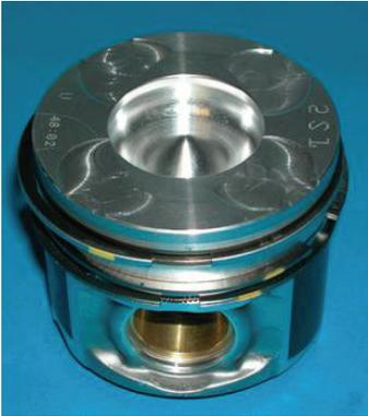
Figure 2.6 View of the piston with the internal bowl
