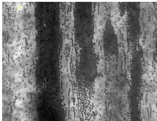
Figure 4.27: Bands of particles at high shear rates.
