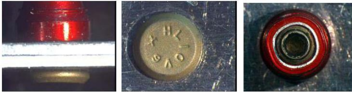
Figure 4.22: Titanium Hi-Lock joint
