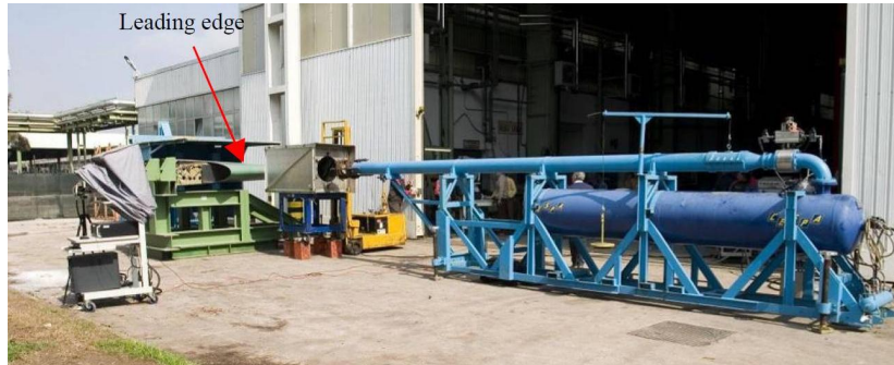
Figure 6.4: Air pressure gun with one single bay leading edge as target
