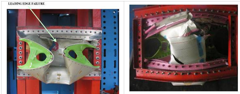
Figure 6.9: Deformed shape of the front and rear view configuration 1
