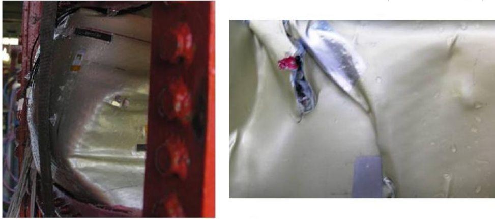
Figure 6.22: Deformation related to the skin inboard (left) and outboard (right)
