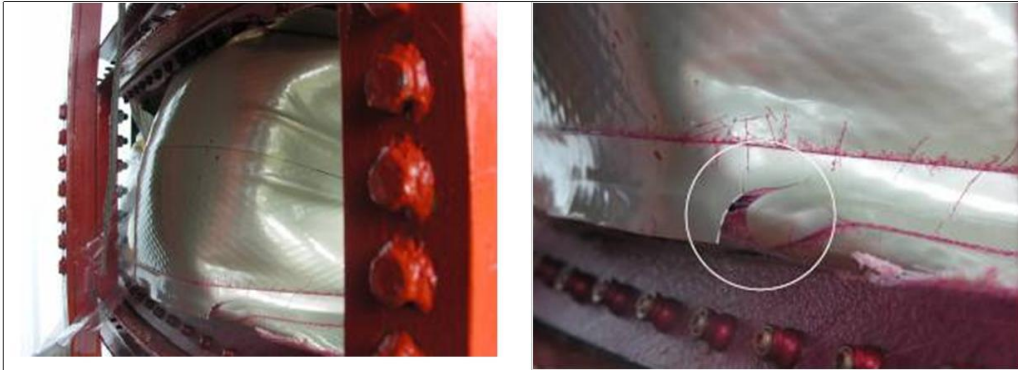
Figure 6.20: Failure zone related to the skin inboard
