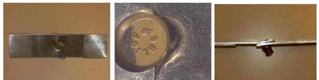
Figure 4.27: Hi-Lock joint after static test
