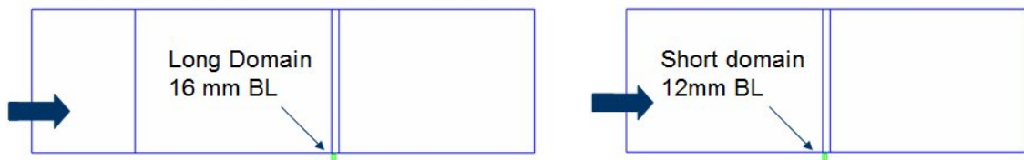
Figure 5-9 The two domains used in order to obtain different BL thickness at the leading edge of the cavity (indicated with the arrow).
