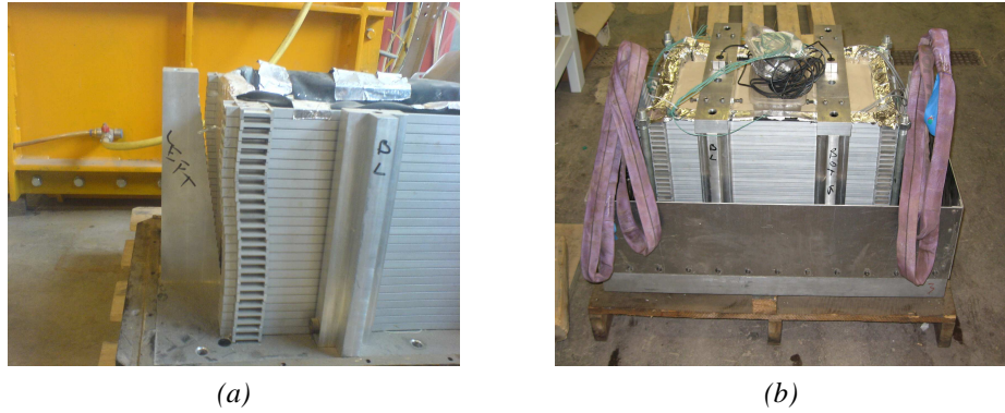
Fig.5.4:Laminar Box; a) Free horizontal displacements; b)Strongbox and base plate
