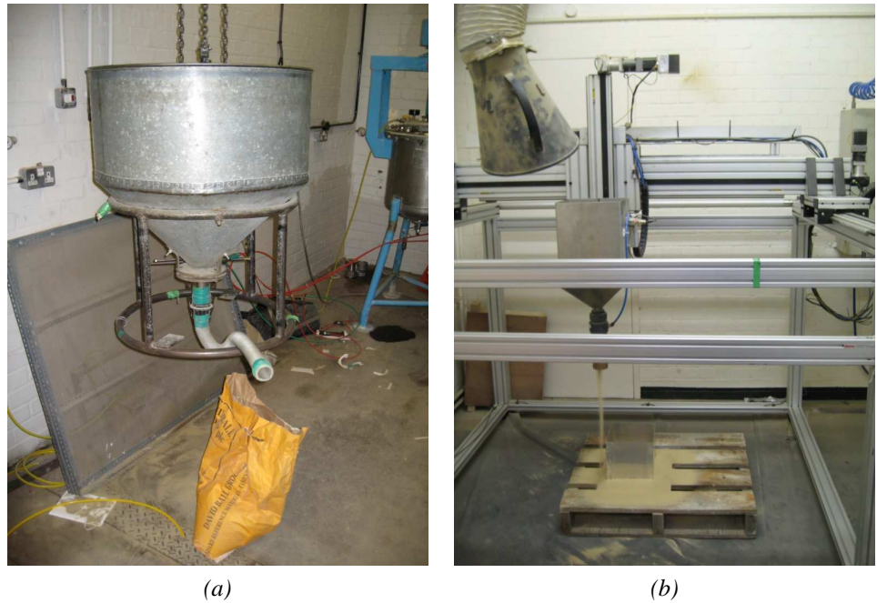
Fig.5.18: Sand pouring: a) hopper for loose sand models; b) automatic sand pourer
