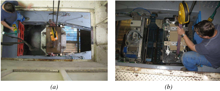
Fig.5.20: Centrifuge loading of a) the counterweight and b) the model
