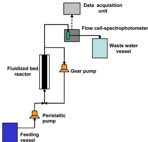
**Fig. 1: Fluidized bed reactor employed for RBBR decolourisation by the means of immobilized laccases**
