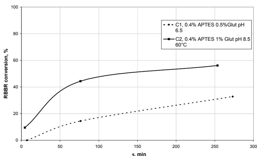
**Fig.6: RBBR conversion degrees plotted versus reactor space-time ( $\tau$ ) . Data refer to decolourisation experiments carried out in fluidized bed reactor operated with immobilized samples C1 and C2.**
