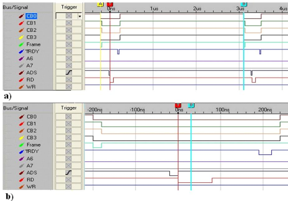
Figure 7.11: Local bus read operation: a) two consecutive reading; b) zoom on the read cycle.
