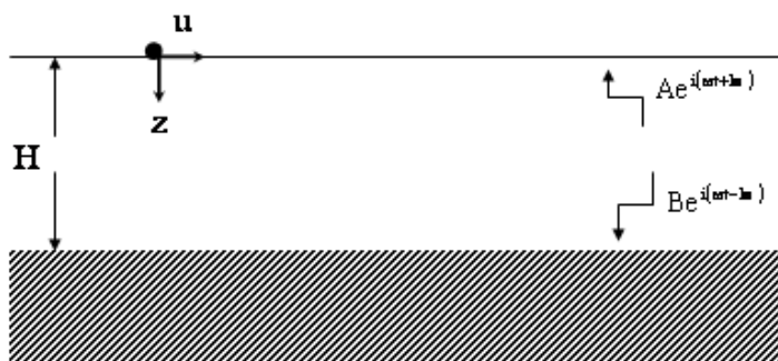
Figure 1.1. Linear elastic soil deposit of thickness H overlying a rigid bedrock.
