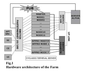
The farm has two independent networks: the first one is used to optimize the data transfer speed among the farm nodes, is split into two subsections, consisting of a Fast Ethernet switch and a Giga Ethernet switch. An uplink connects these two switches to implement an equivalent single private network. The two private network subsections are necessary because the Super Micro nodes have Fast Ethernet links, while the APPRO ones have Giga Ethernet links.
