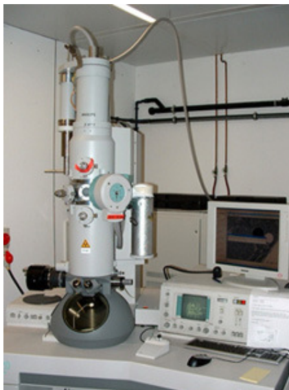
Figure 7.1: Picture of the cryo-electron microscope used, a Philips CM120 BioTWIN operating at 120 kV.
