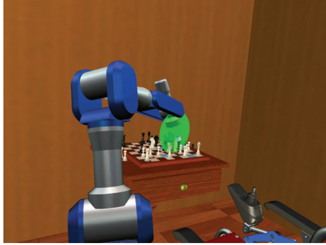
Figure 3.10: The manipulability ellipsoid during the task execution.
