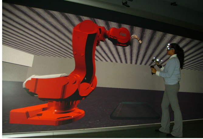
Figure 3.9: The kinematic chain being dragged by the virtual hand.
