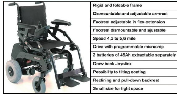
Figure 4.3: The real Neatech Indoor wheelchair is lightweight and powered
