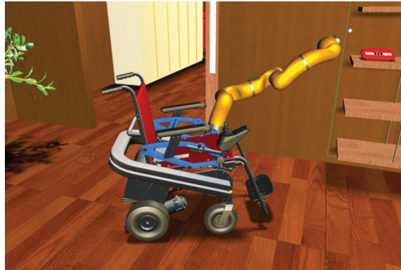
Figure 4.2: The virtual environment with a wheelchair-mounted manipulator on a sliding rail
