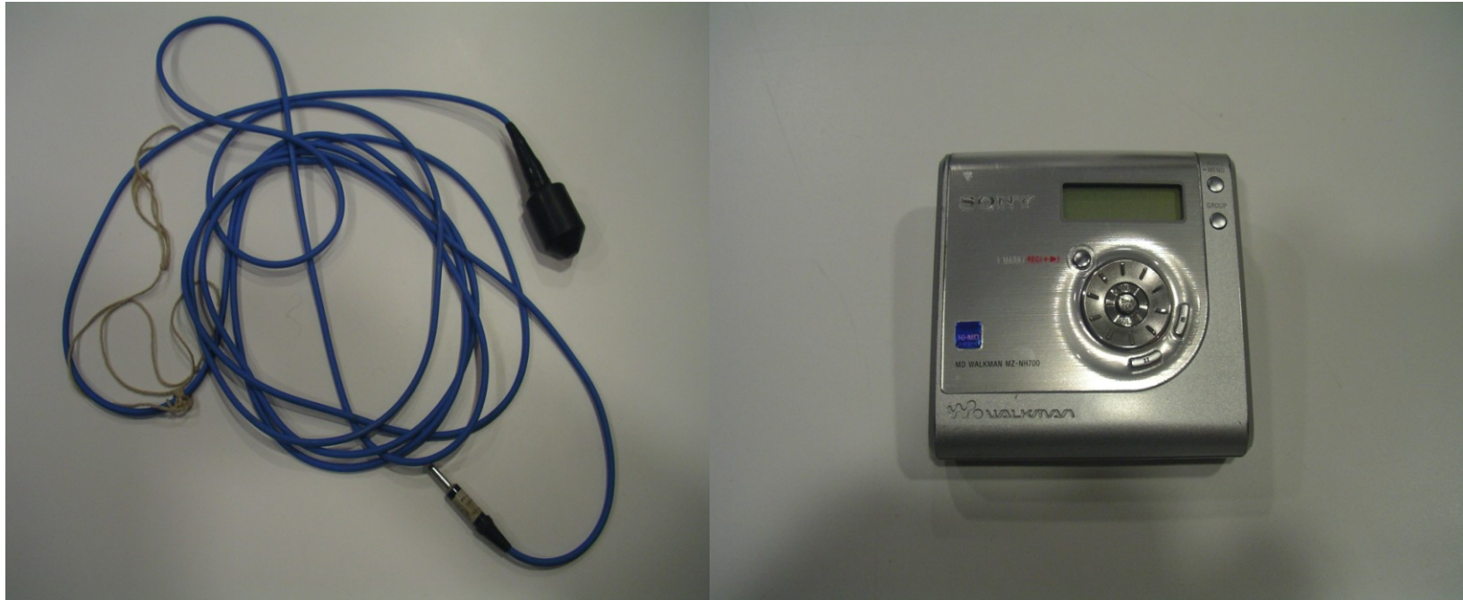
Fig 2.3: PZ-1A hydrophone (left) and MZ-NH700 Sony digital audio disk (right) used to record vocalisations of common dolphins ( Delphinus sp.) in the Hauraki Gulf, New Zealand between February 2008 and May 2009 (photo by Author)
